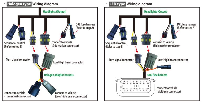
A Connect DRL fuse harness to the lights, then insert the fuse into fuse box.
