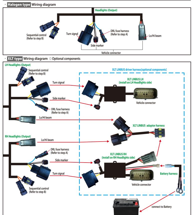
A Connect DRL fuse harness to the lights, then insert the fuse into fuse box.
